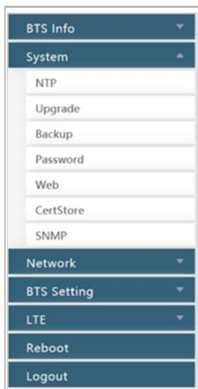
The *System* menu for BaiBS\_QRTB\_2.6.2 includes Network Time Protocol (NTP), software upgrade/rollback, configuration backup, password reset (for the eNB GUI), diagnostics, and the CertStore for uploading eNB certificates, e.g., licensing files. See Figure 2-13.
