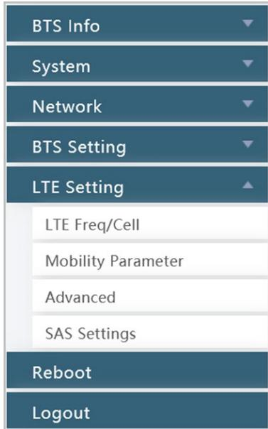
Use the first 3 sub-menus under the *LTE Setting* menu to (a) configure the neighboring eNBs' frequencies and identify each eNB running on that frequency ([section 2.10.1](#)); (b) configure the current eNB's mobility parameters (beginning with [section 2.10.2](#)); and (c) examine the current eNB's advanced settings ([section 2.10.4](#)).
