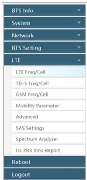
Use the first 5 sub-menus under LTE to (a) configure the neighboring eNBs' frequencies and identify each eNB running on that frequency ([section 2.9.1](#)); (b) configure the current eNB's mobility parameters (beginning with [section 2.9.2](#)); and (c) examine the current eNB's advanced settings ([section 2.9.6](#)).
