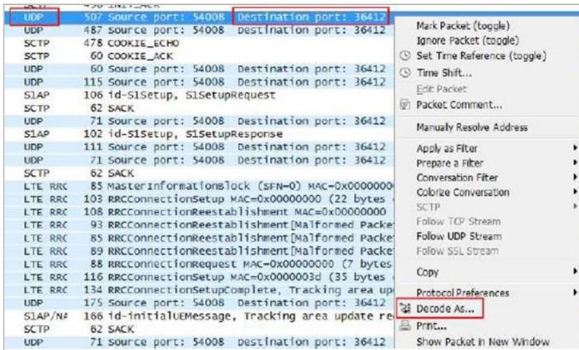
3. Go to the *Transport* tab, and set the destination as 36412 and the decoding type as SCTP (Figure 2-93). Get the SCTP message as shown in the figure.
