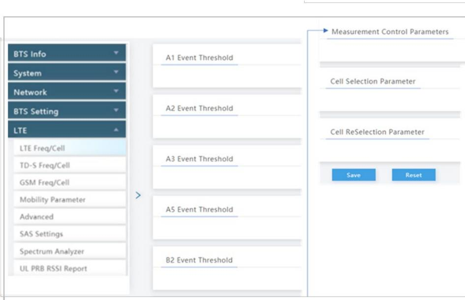
Figure 2-72: A1, A2, A3, and A5 Event Thresholds (RTS/RTD)
