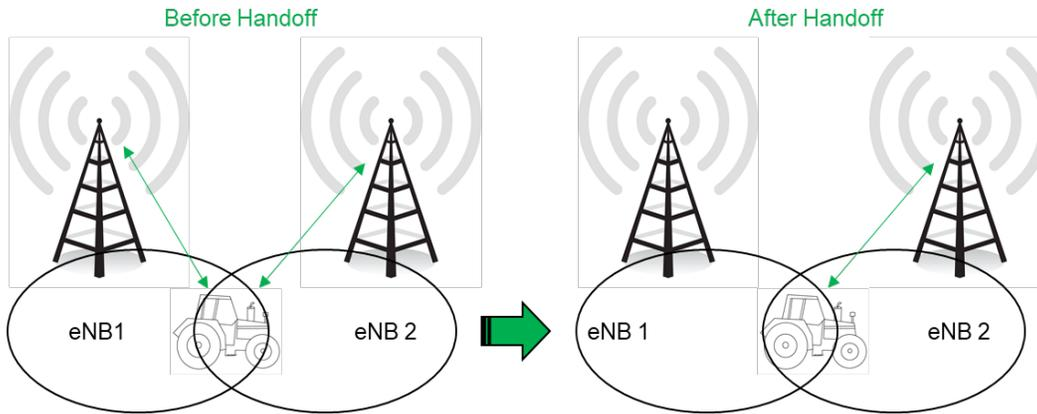
What the UE measures that determines cell selection and reselection is the Reference Signal Received Power (RSRP) of the serving as well as neighboring eNBs. The measurements are sent periodically to the serving eNB, which then determines if the UE would be better served by an adjacent eNB. Refer to the case study in [section 2.11 Real-World LTE to LTE Handoff Configuration Example](#).
