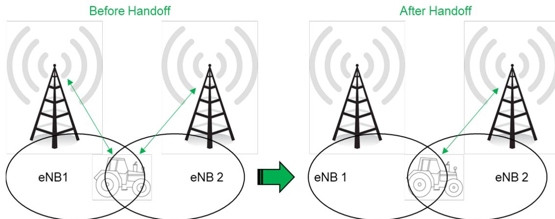
What the UE measures that determines cell selection and reselection is the Reference Signal Received Power (RSRP) of the serving as well as neighboring eNBs. The measurements are sent periodically to the serving eNB, which then determines if the UE would be better served by an adjacent eNB. Refer to the case study in [section 2.11 Real-World LTE to LTE Handoff Configuration Example](#).
