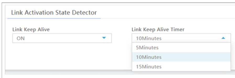
The screenshot shows a configuration window titled "Link Activation State Detector". It contains two dropdown menus. The first is labeled "Link Keep Alive" and has "ON" selected. The second is labeled "Link Keep Alive Timer" and has a list of options: "10Minutes", "5Minutes", "10Minutes", and "15Minutes". The "10Minutes" option is currently selected.
