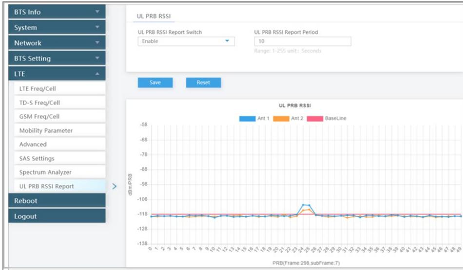
Figure 2-110: LTE > UL PRB RSSI Report (With Interference) (RTS/RTD)
