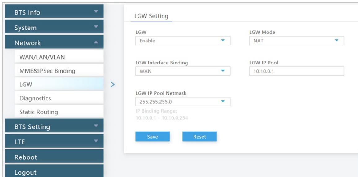
The screenshot displays the 'LGW Setting' configuration page. On the left is a navigation sidebar with categories: BTS Info, System, Network (expanded), BTS Setting, LTE, Reboot, and Logout. Under 'Network', 'LGW' is selected. The main panel shows the following settings:
